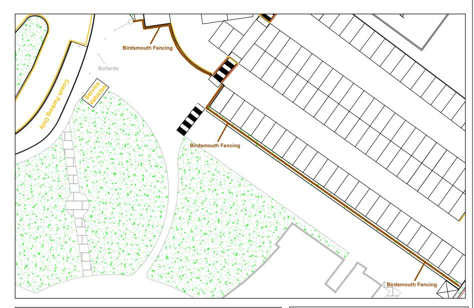
Installation of access control Barrier to control overflow parking, bollards and single rail timber fence following the kerb line to secure area and prevent parking on pavement. Inclusion of zebra crossing for pedestrians safety across the access road.
